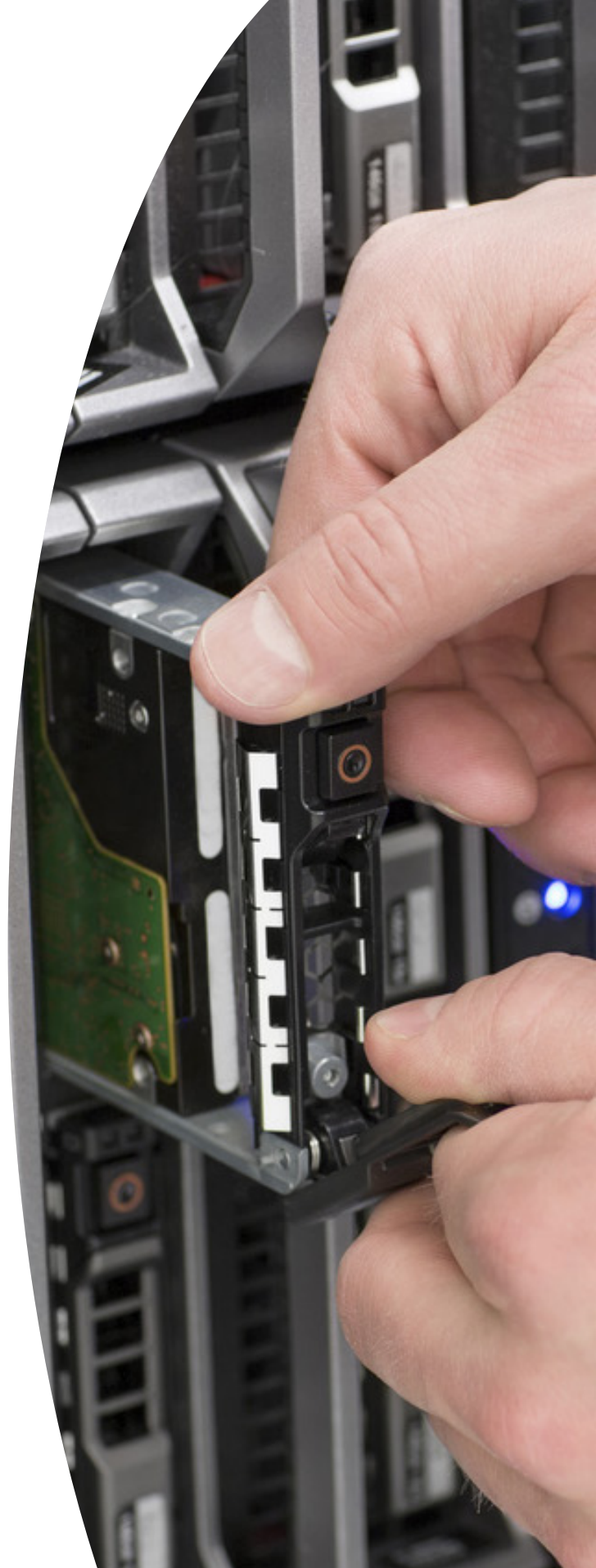
Inserting Hard Drive into PowerEdge Modular Blade server
